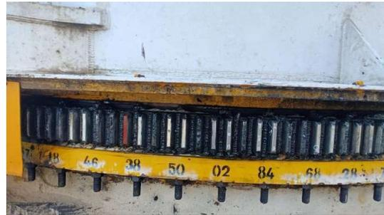
Gambar 2. Slewing gear.
