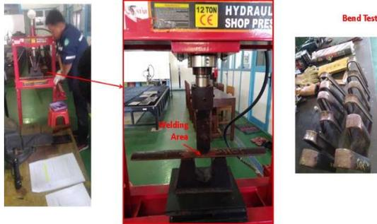
Gambar 5. Proses uji bending.
