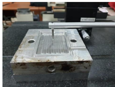
Figure 2. The design of mold cavity for pre-designed of microchannel chip.
