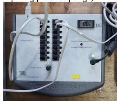
**Gambar 3.** Digital strain display
