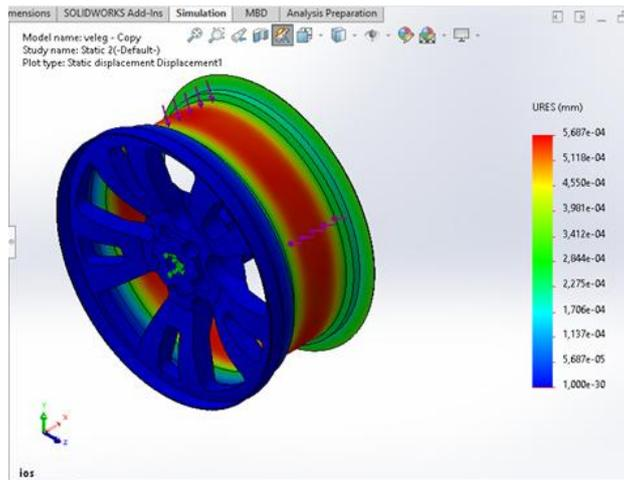
Figure 7. Displacement analysis
