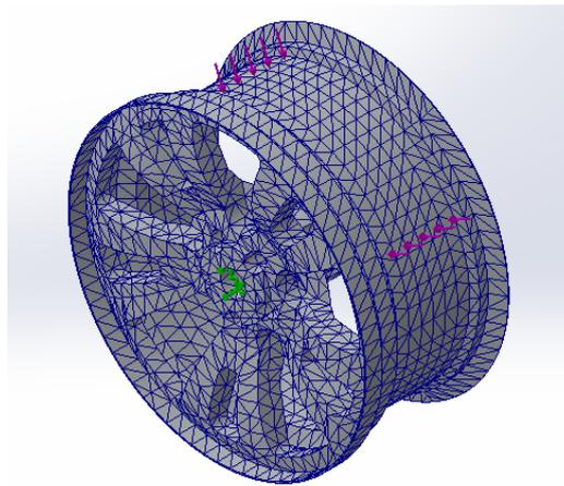
**Figure 3.** Meshing process
