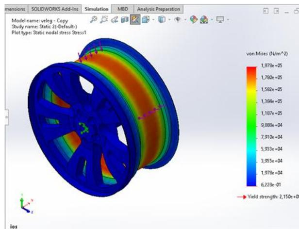
Figure 5. Von mises stress
