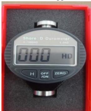
Gambar 9. Alat Uji Kekerasan Shore Durometer Digital
