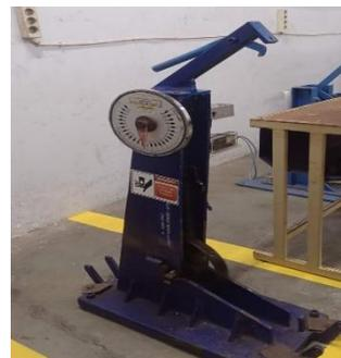
Gambar 8. Alat Uji Impact Charpy Test
