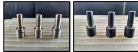
a. Raw Material b. Pack carburizing
