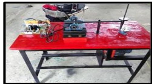
Gambar 1. Tribometer Pin - On - Disc
